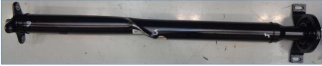
Figure 11 Buckling mode of the experimental test of Sample 1
