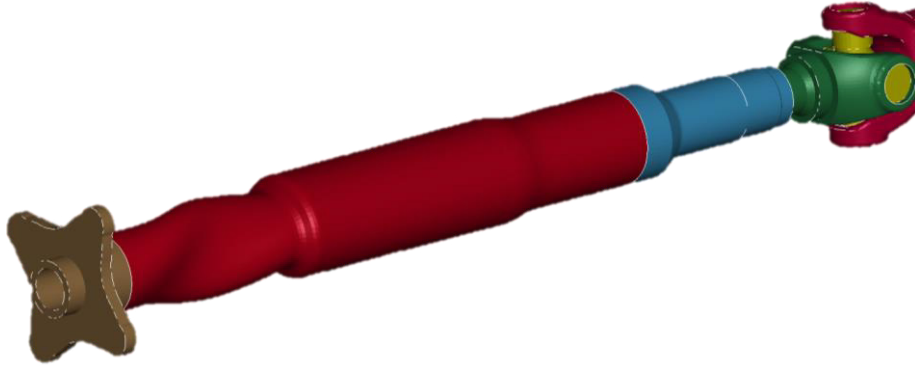
Figure 14 Detailed visualization of the torsional buckling mode
